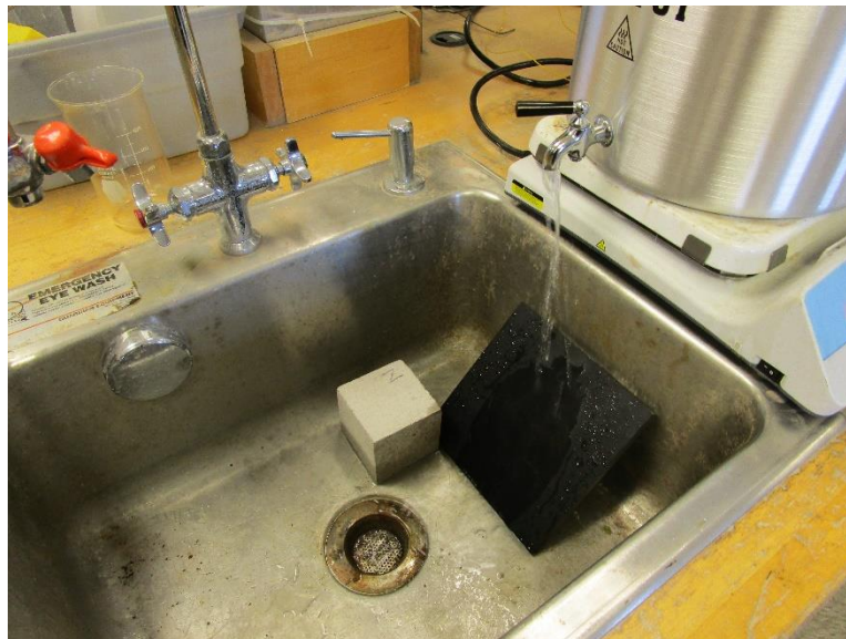
Photo No. 8 SEFA 8 - Hot Water Test
