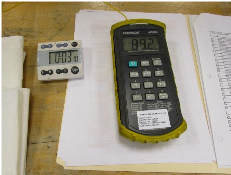
Photo No. 10 SEFA 8 - Hot Water Test
