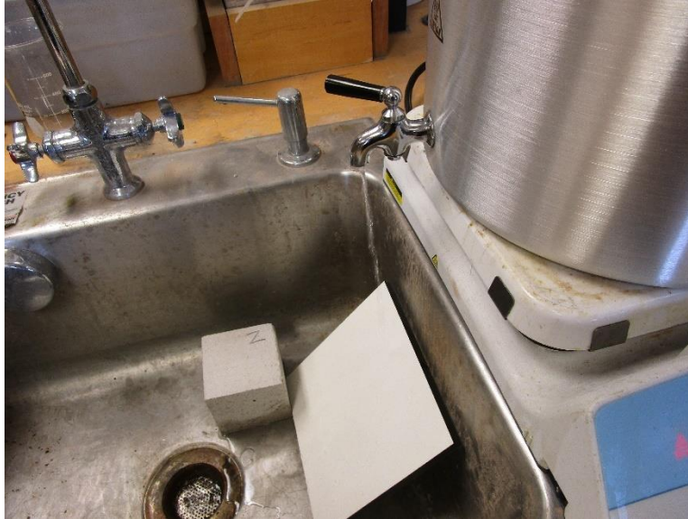
Photo No. 9 SEFA 8 - Hot Water Test
