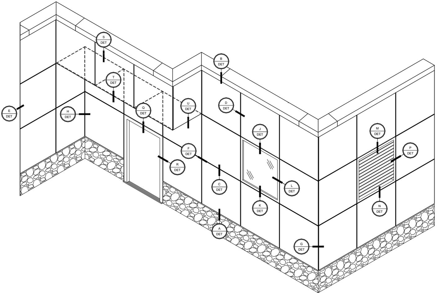
Extruded aluminum furring must be attached to structural members designed to support the dead and live loading of the entire wall system. The following details do not specify, suggest, or imply the attachment between the structure and aluminum furring. The customer is responsible for the structural engineering of attachment to structure.
